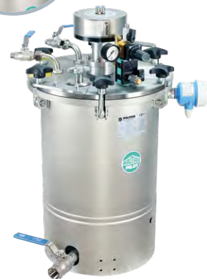
MDG 45 KLA with air-driven type 46-735 agitator along with tuning fork sensor to protect against overfilling. Fill at the bottom valve. The two upper valves for material recirculation - feed and return.
