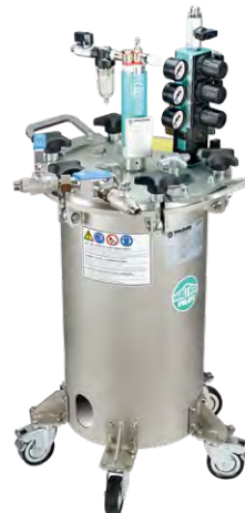
MDG 22 KLA with air-driven type 46-810 agitator, air inlet fittings with two additional regulators, as well as splitter with two ball valves to connect two spray guns. The tank is equipped with castors and hand grips for portable use.
